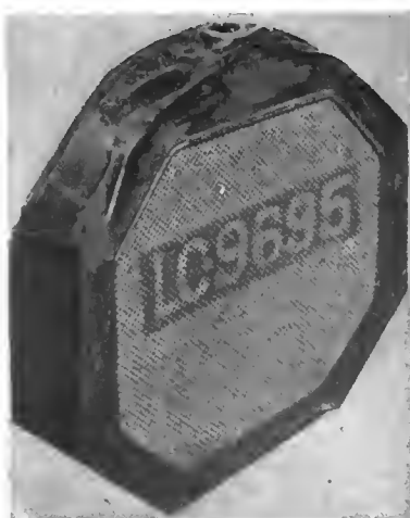
FIG. 8.—Radiator that withstood overturn of car. The tubes were uninjured.
